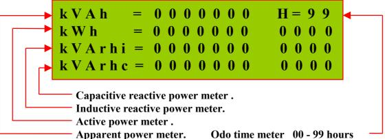
*NOTE:* If device has internal current transformer of 5 A and (Current Transformer Ratio) CT=5000/5, values on the screen comes out as a VAh,Wh, VArhi and VArhc, even written unit on the device kVAh, kWh, kVArhi and kVArhc.
