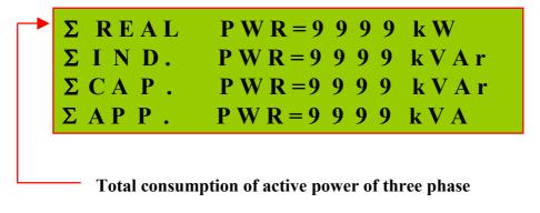
*NOTE:* If device has internal current transformer of 5 A and (Current Transformer Ratio) CT=5000/5, values on the screen comes out as a W, even written unit on the device kW.
