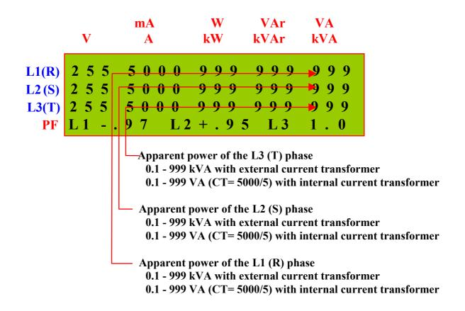
Also as below you can find total consumption of apparent power of three phases on the 4.line of the 2. page of the main menu .
