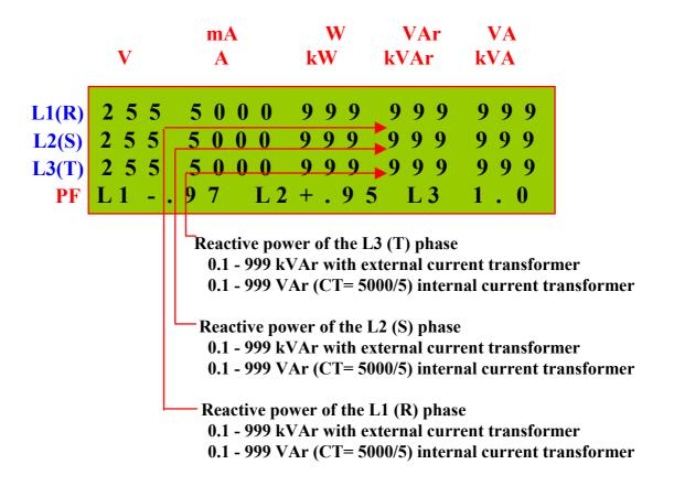
NOTE: To determine the reactive power if capacitive or inductive, sign of power factor of each phase indicates that moment. If the sign is (-) means capacitive reactive power, other wise (+) inductive reactive power. Also as below you can find total consumption of reactive power of three phases on the 2. and 3.line of the 2. page of the main menu.
